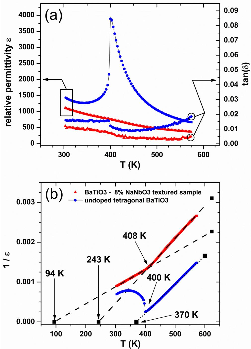
**Fig. 3:** BaTiO<sub>3</sub> – 8% volume NaNbO<sub>3</sub> textured sample and tetragonal "pure" BaTiO<sub>3</sub> ceramic (color online): (a) relative permittivity and dielectric losses versus temperature (1 MHz), (b) reciprocal relative permittivity versus temperature (Curie-Weiss law, 1 MHz).
