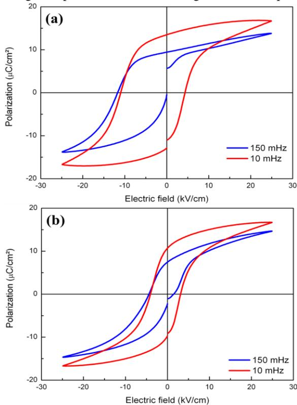
Fig. 4. Hysteresis loops measured at 150 mHz and 10 mHz of (a) cobalt doped BaTiO<sub>3</sub> and (b) niobium and cobalt co-doped BaTiO<sub>3</sub>.
