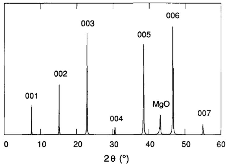
**Fig. 1.** X-ray diffraction pattern of YBCO film showing its (001) orientation.
