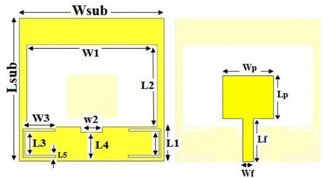
Fig. 2. (a) The proposed UWB slot antenna schematic.
