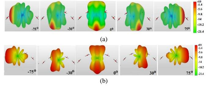
Figure 8. Beam-steering situations of the selected phased array, (a) Far-field radiation patterns, (b) Near-field radiation pattern.
