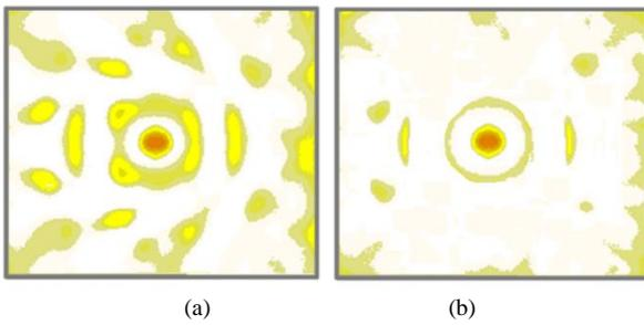
Figure 9. Imaging result achieved by (a) the rectangular antenna array, and (b) the round antenna array.
