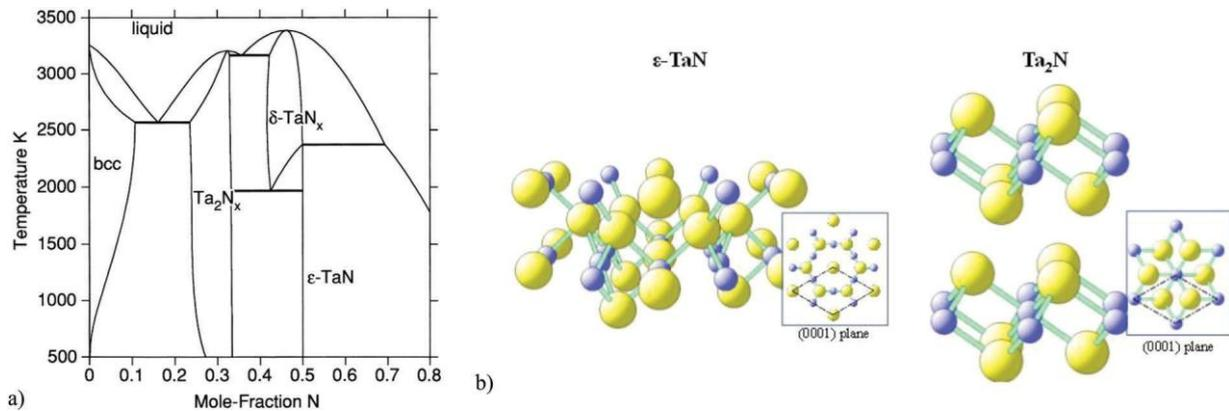
Figure 3. a) Phase diagram of the Ta–N system<sup>[68,69]</sup> (Reproduced with permission.<sup>[69]</sup> Copyright, Springer); b) crystalline structures of  $\epsilon$ -TaN ( $P6/mmm$ ) and  $Ta_2N$  ( $P\bar{3}m$ ): N and Ta: blue and yellow spheres, respectively; dashed lines in the insets indicate the cell unit (Reproduced with permission.<sup>[72]</sup> Copyright, American Physical Society).
