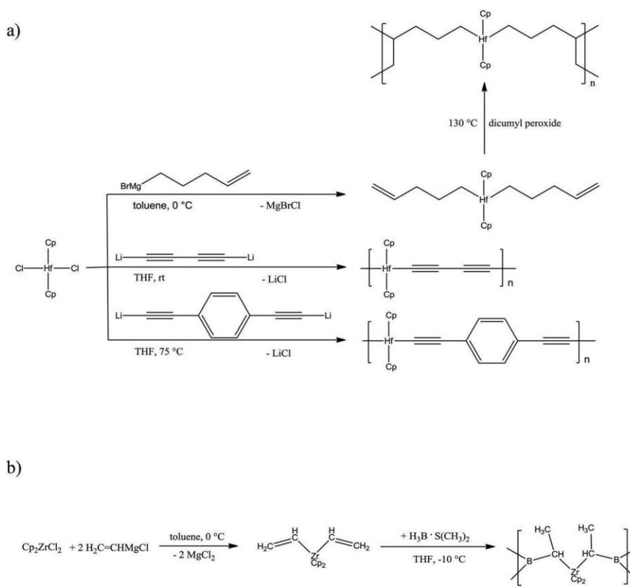
Figure 11. a) Synthesis of non-oxidic preceramic polymers for  $\text{HfC}$  starting from  $\text{Cp}_2\text{HfCl}_2$ <sup>[125]</sup>; (b) synthesis of  $\text{ZrC}/\text{ZrB}_2$  using a preceramic polymer synthesized from a divinyl-substituted zirconocene and borane.<sup>[126]</sup>
