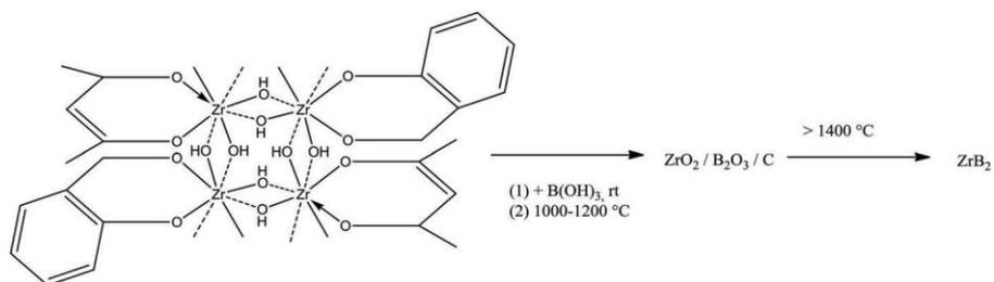
Figure 9. a) Synthesis of  $\text{ZrB}_2$  upon high thermal conversion of  $\text{B}(\text{OH})_3$ -modified polyzirconoxanes in argon atmosphere.<sup>[123]</sup>
