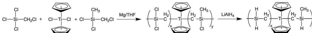
Figure 20. Two-step synthesis of a polymeric single-source precursor containing Ti and Si mixed at molecular scale.<sup>[195]</sup>
