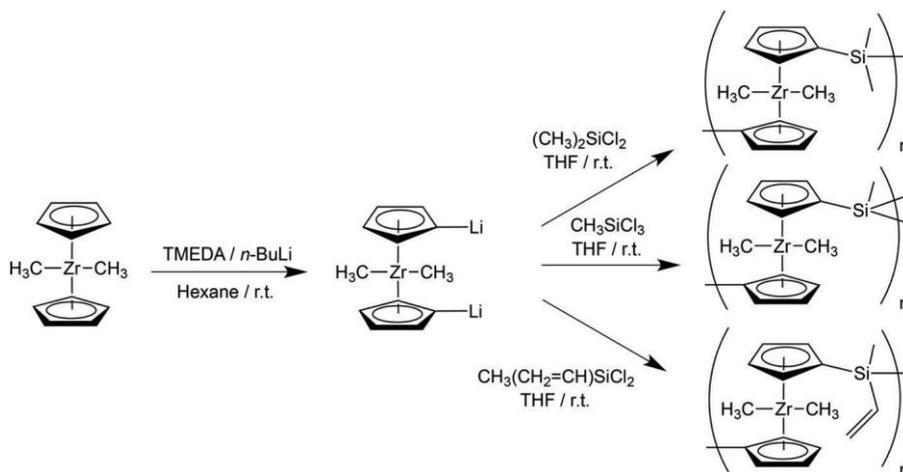
Figure 21. Synthesis of preceramic polymers via the reaction of dilithiozirconocene complex with various chlorosilanes.<sup>[196]</sup>
