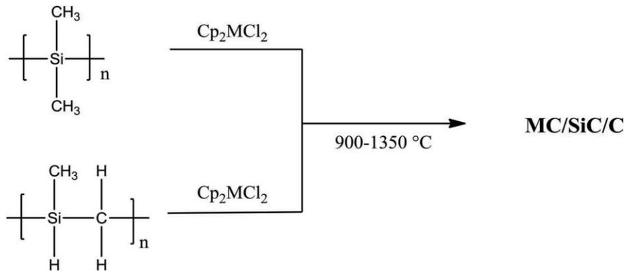
Figure 13. Synthesis of MC/SiC/C nanocomposites ( $M \frac{1}{4}$  Ti, Zr, Hf) from polydimethylsilane or polymethylhydridocarbosilane modified with metallocene dichlorides ( $Cp \frac{1}{4}$  cyclopentadienyl).<sup>[143]</sup>
