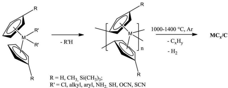
Figure 10. Use of sandwich metal complexes ( $\text{M}_{1/4}\text{Ti}, \text{Zr}, \text{Hf}$ ) as precursors for the synthesis of  $\text{MC}_x/\text{C}$  nanocomposites. Their thermal decomposition was shown to occur via formation of polymeric intermediates.<sup>[124]</sup>
