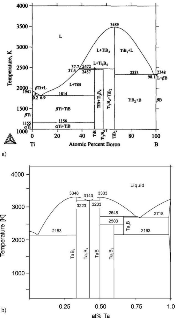
Figure 1. Phase diagrams of a) Ti-B (<http://www.calphad.com/titanium-boron.html>) and b) Ta-B systems. Reproduced with permission.<sup>[20]</sup> Copyright, Elsevier.
