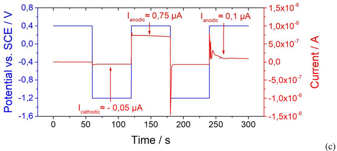
**Figure 8-** Electrochemical activation of an artificial defect
