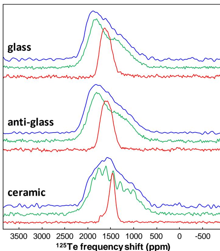
**Figure 10.**  $^{125}\text{Te}$  NMR spectra recorded at 7 T for the glass (top), anti-glass (middle) and ceramic (bottom) BNT samples. In blue: static spectrum; in green: MAS spectrum (MAS frequency of 14285 Hz); in red: isotropic spectrum obtained from the PASS experiment (see SI-5 for the 2D spectra).
