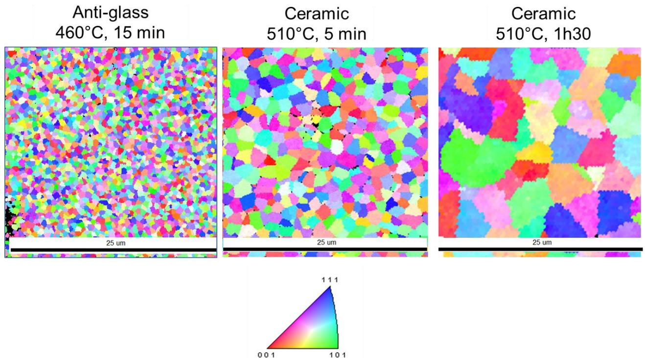
**Figure 2.** EBSD of BNT parent glass heat-treated at 460°C, 15 minutes; 510°C, 5 minutes and 510°C, 1h30 (scale bar: 25 μm).
