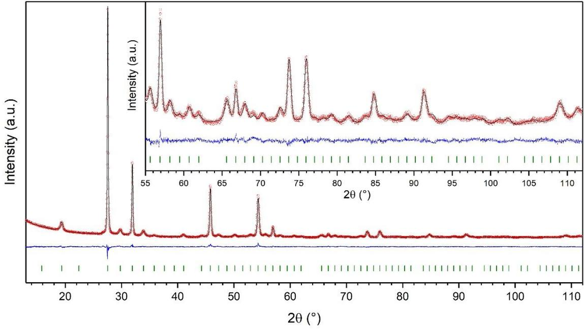
**Figure 6.** Experimental (red circles), fitted (black solid line) and difference curve (blue solid line) of the XRD Rietveld diagram refinement of the  $\text{Bi}_{0.8}\text{Nb}_{0.8}\text{Te}_{2.4}\text{O}_8$  ceramic material. The inset corresponds to an enlargement of the same refined data. Reliability factors are  $R_B = 4.38\%$ ,  $R_F = 2.37\%$ ,  $\chi^2 = 2.47$ .
