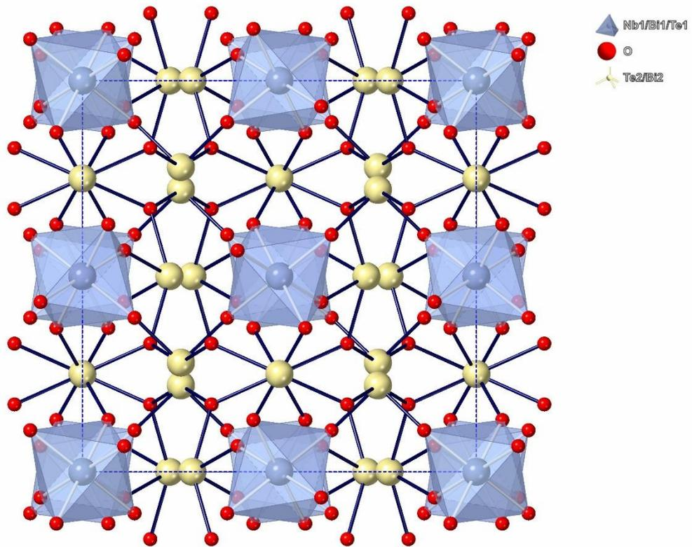
**Figure 8.** Schematic [001] view of the  $\text{Bi}_{0.8}\text{Nb}_{0.8}\text{Te}_{2.4}\text{O}_8$  ceramic structure. The blue, white and red spheres denote mixed Bi1/Nb1/Te1, Bi2/Te2 and O atoms, respectively.[16]
