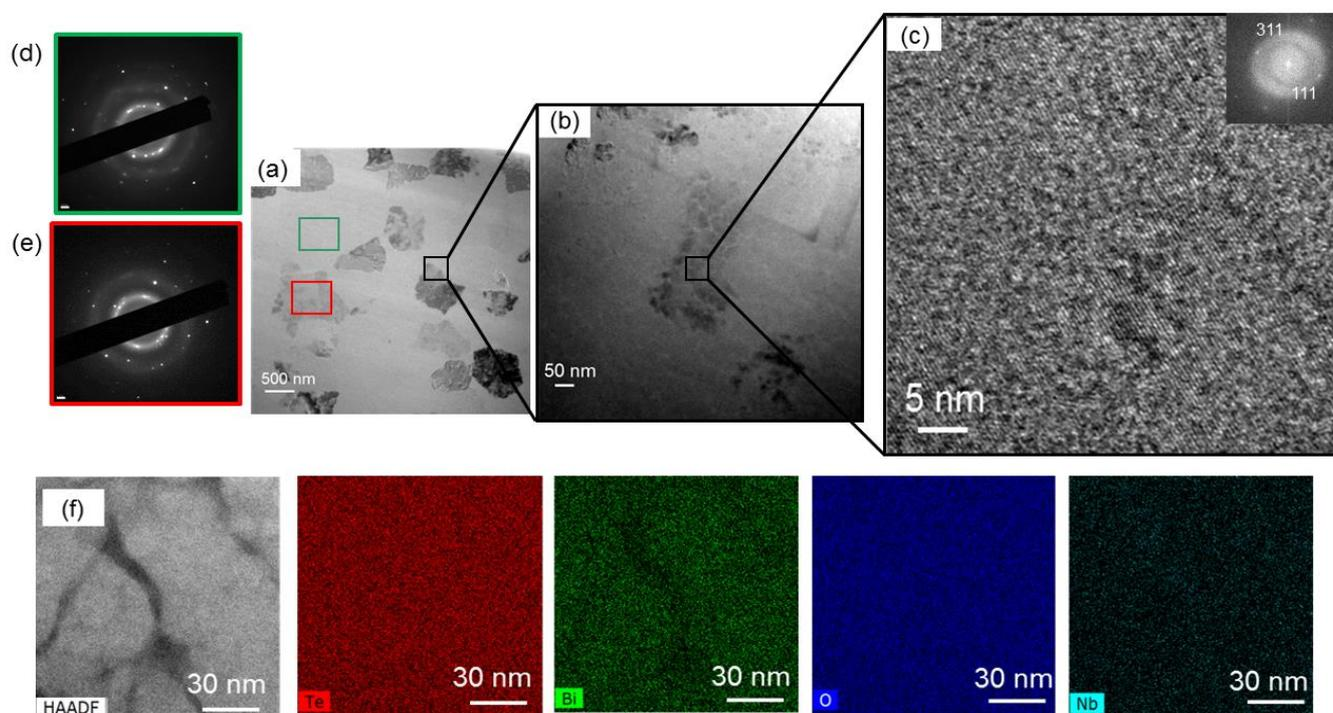
**Figure 12.** BNT anti-glass 460°C 15 min (a), (b) Bright Field TEM micrographs of the multiscale microstructure, (c), HRTEM image and corresponding FFT pattern showing the complex mixing between amorphous and crystalline areas, (d), (e) Selected Area Electron Diffraction patterns of the light and dark grey areas respectively (f) STEM-HAADF image (Z-contrast) and STEM-EDX elemental maps highlighting a Bi depletion grains.
