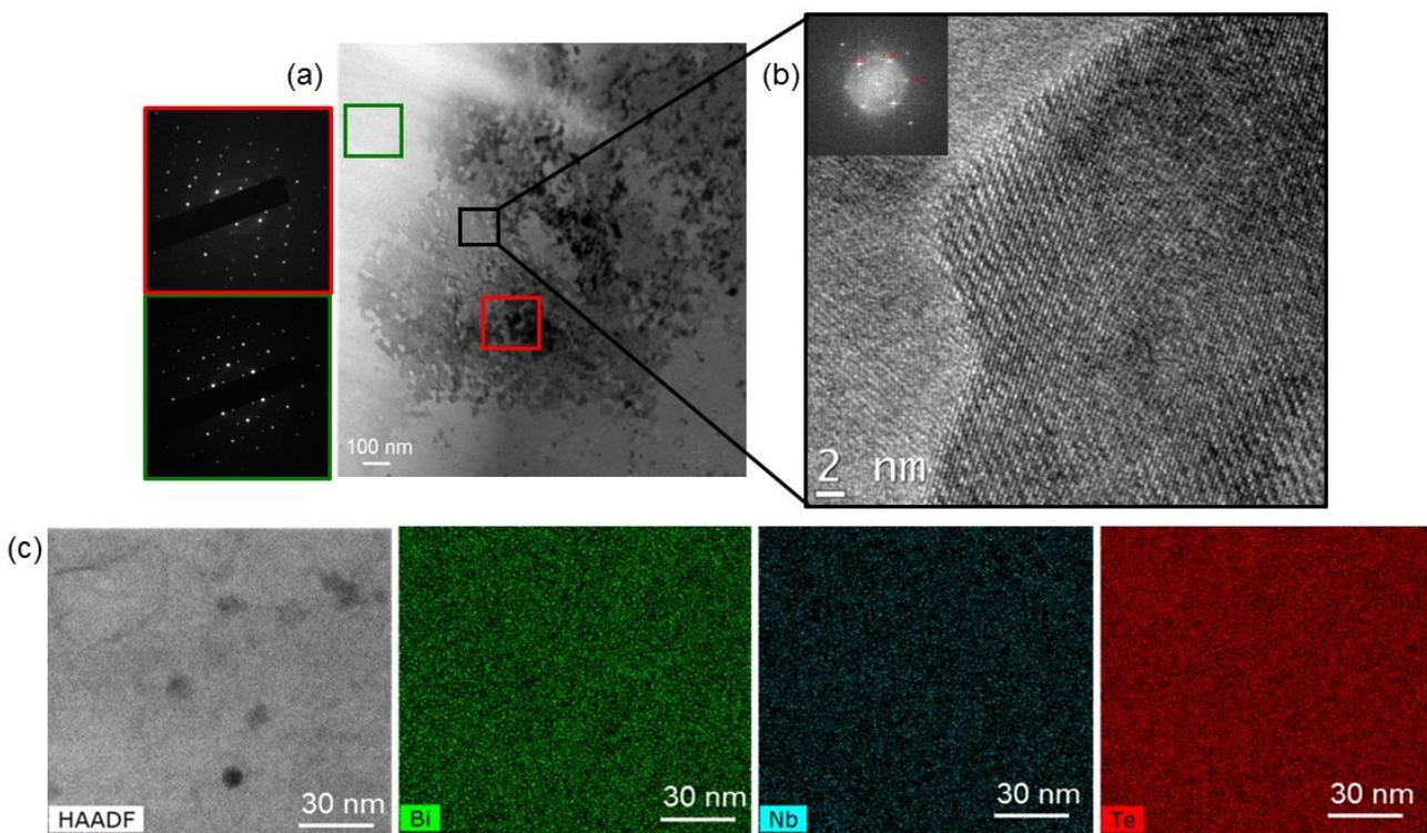
**Figure 13.** BNT ceramic 510°C 5 min (a) Bright Field TEM micrograph showing large domains constituted of smaller grains and corresponding Selected Area Electron Diffraction patterns, (b) HRTEM image exhibits crystalline plans and narrow grain boundary, (c) STEM-HAADF image (Z-contrast) and STEM-EDS elemental maps showing a better chemical homogeneity compared to the anti-glass (Figure 12).
