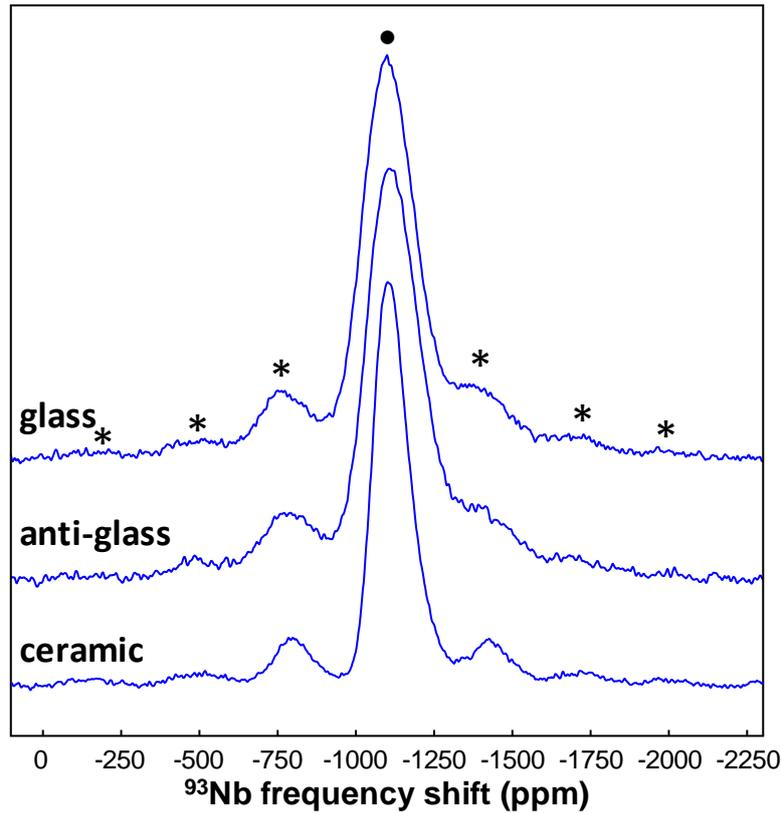
**Figure 9.**  $^{93}\text{Nb}$  MAS NMR spectra (in blue) recorded at 20 T with a MAS frequency of 65 kHz for the glass (top), anti-glass (middle) and ceramic (bottom) BNT samples. The full circle and the stars denote the isotropic line and the spinning sidebands of the central transition, respectively (see SI-4 for the reconstructed spectra).
