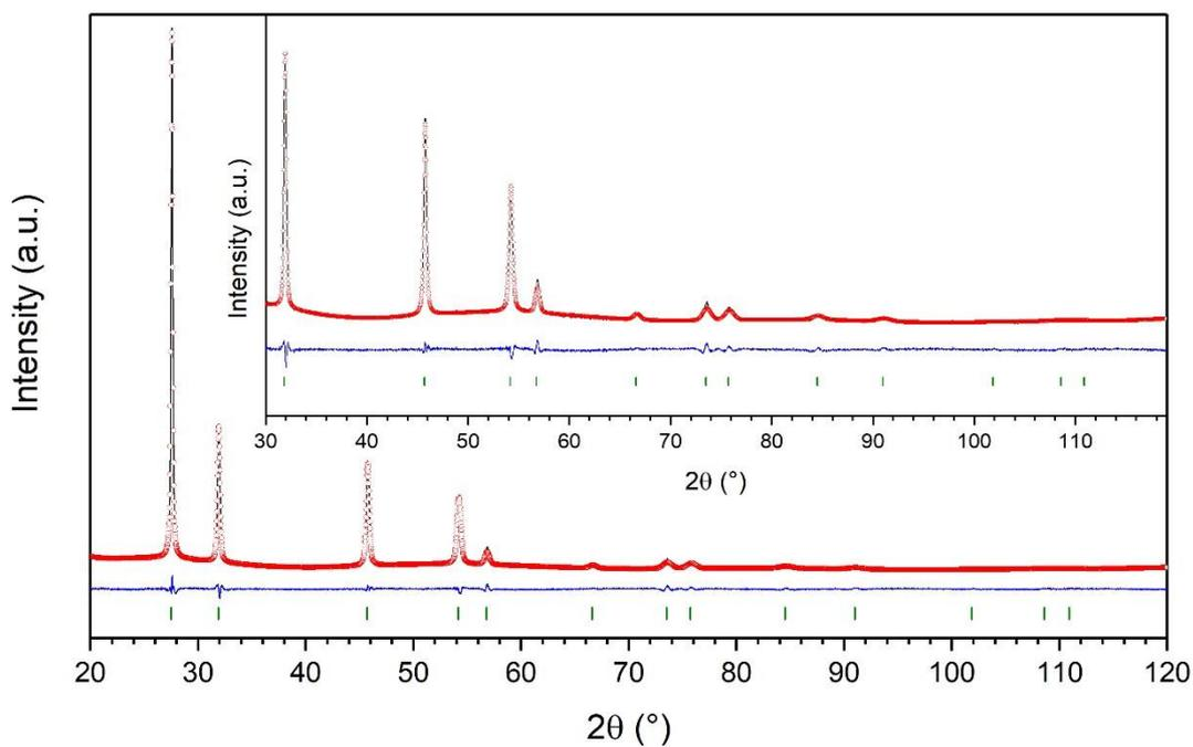
**Figure 4.** Experimental (red circles), fitted (black solid line) and difference curve (blue solid line) of the XRD Rietveld diagram refinement of the  $\text{Bi}_{0.8}\text{Nb}_{0.8}\text{Te}_{2.4}\text{O}_8$  anti-glass material using a site splitting model for the oxygen position (192l site). The inset corresponds to an enlargement of the same refined data. Reliability factors are  $W_{Rp} = 4.87\%$ ,  $GOF = 1.59$ ,  $R_p = 3.70\%$ .
