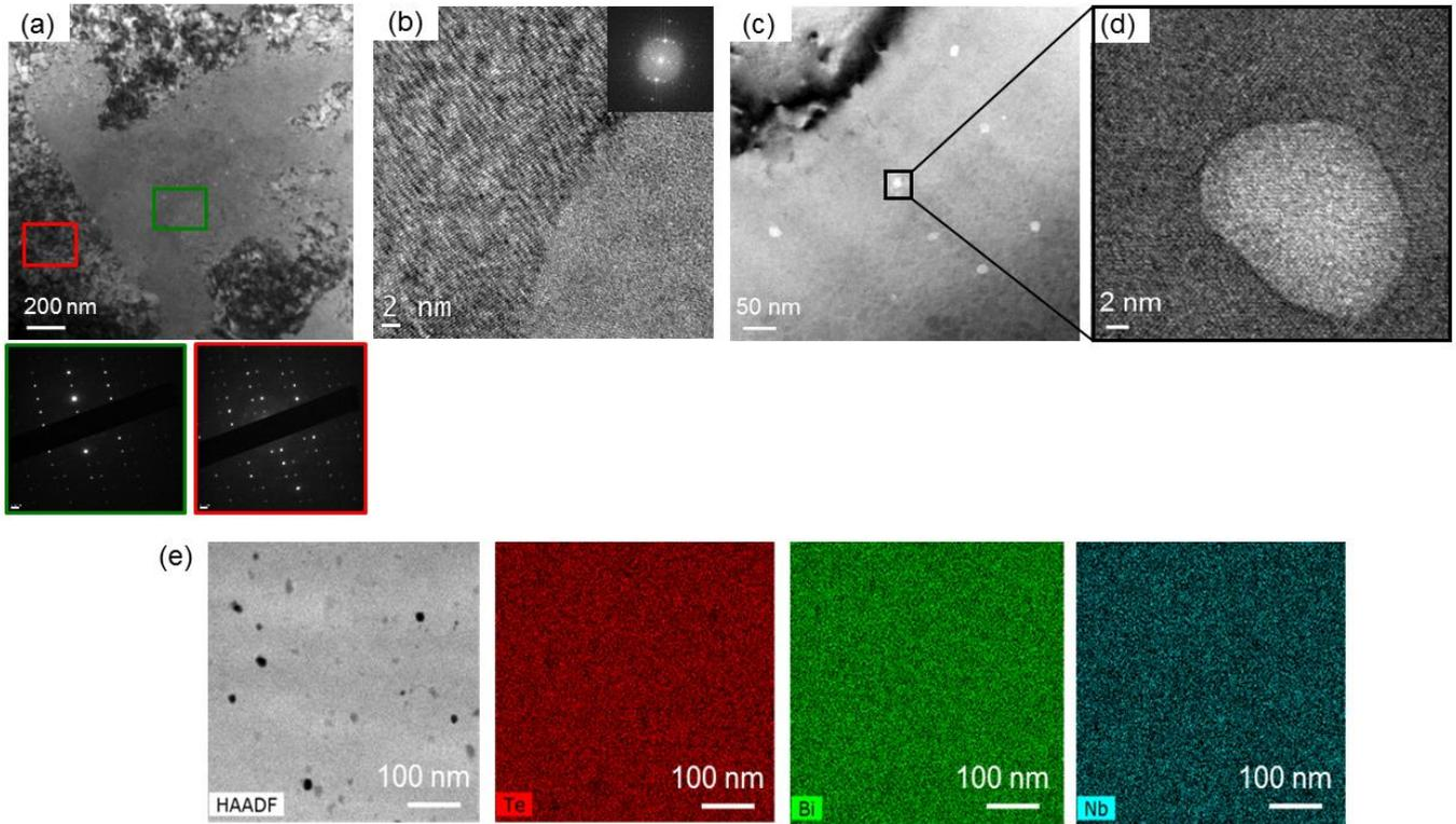
**Figure 14.** BNT ceramic 510°C 1h30 (a) (b) Bright Field TEM and HRTEM micrographs showing large domains constituted of smaller grains and corresponding Selected Area Electron diffraction patterns, (c) (d), Bright Field TEM and HRTEM micrographs of porosity, (e) STEM-HAADF image (Z-contrast) and STEM-EDS elemental maps showing a better chemical homogeneity compared to the anti-glass (Figure 12).
