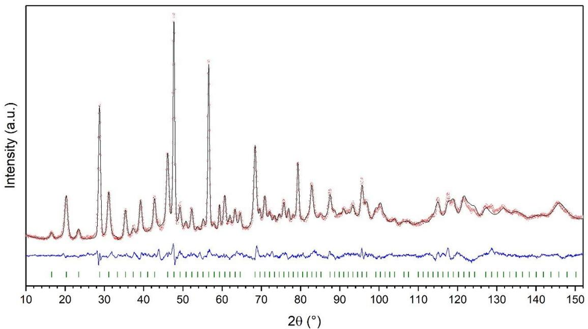
**Figure 7.** Experimental (red circles), fitted (black solid line) and difference curve (blue solid line) of the NPD Rietveld diagram refinement of the  $\text{Bi}_{0.8}\text{Nb}_{0.8}\text{Te}_{2.4}\text{O}_8$  ceramic material. Reliability factors are  $R_B = 4.45\%$ ,  $R_F = 3.01\%$ ,  $\chi^2 = 6.62$ .
