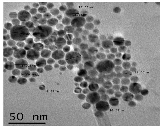
Figure 2: TEM images of gold nanoparticles (AuNP@PEI) with ratio (m<sub>PEI</sub>/m<sub>Au</sub> = 0.46)
