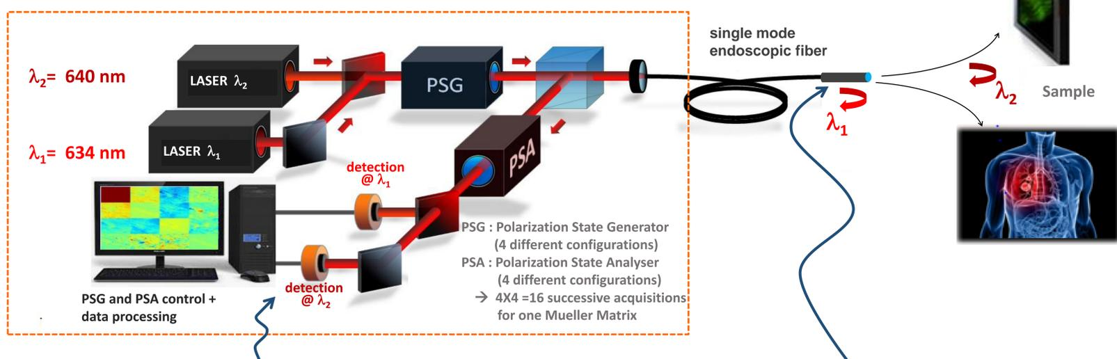
**Two-wavelength differential method (TWDM) based on a simultaneous measurement at two close wavelengths [2]**
