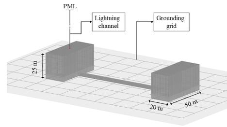
Fig. 1. Calculation model of the reference case.
